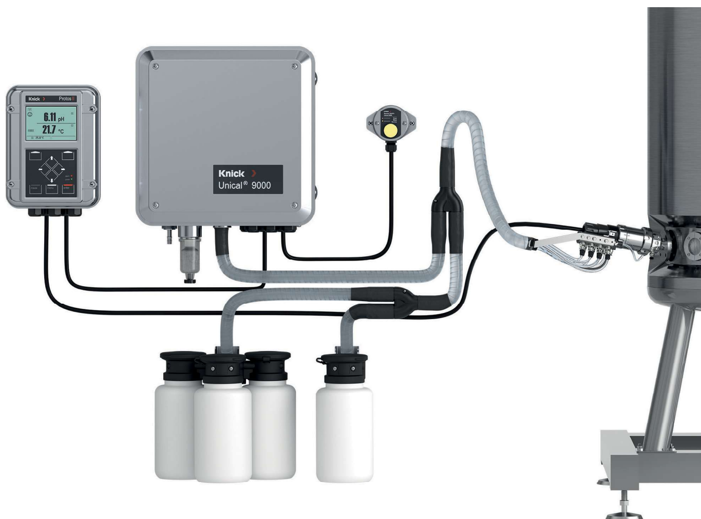
cCare pHarma: Automated, standardised cleaning and calibration of pH sensors for reliable measurements at all times. Audit trail transmission via fieldbus is available independently of cCare. When cCare is used, additional maintenance and calibration activities can be incorporated into the same digital information flow.
