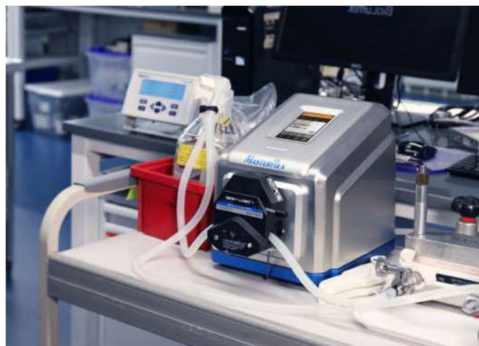
Peristaltic pump system with tubing setup for precise fluid transfer
