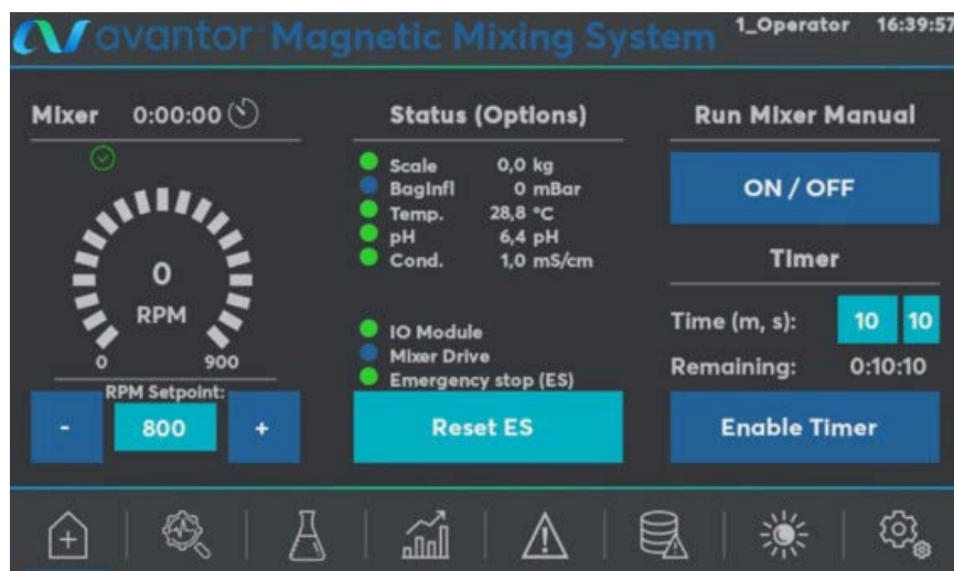
FIGURE 1: The Avantor Magnetic Mixer system touchscreen interface is designed for simplicity and consistency across all mixer sizes. The unified layout provides clear visibility of key parameters such as rpm, temperature, pH, conductivity, and scale weight, along with intuitive controls for manual operation and timers. By maintaining the same interface from development to production systems, operators can easily transition between scales without additional training, reducing complexity and improving process efficiency.
