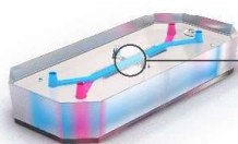
Figure 1: Diagram of an Organ-Chip. The original Organ-Chip design, Chip-S1 Stretchable Chip, consists of two parallel microfluidic channels (1, 6), with distinct channels for epithelial cells (2) and endothelial cells (5) and their respective cell culture media. A porous membrane (4) separates the two channels while enabling inter-channel communication and cell migration. Vacuum channels (3) alongside the microfluidic channels provide tunable mechanical stretch across the membrane. Image credit: Emulate, Inc.
