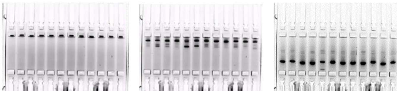
Figures 1–3: DNA migration through a gel cassette illustrating synchronised arrival at the extraction wells using Ranger Technology (Yourgene Health).
