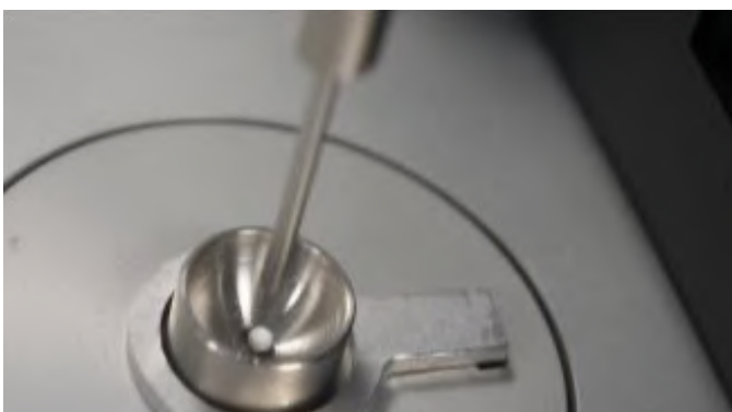
Figure 6: The MicroPress indenter pressing down onto a lyobead
